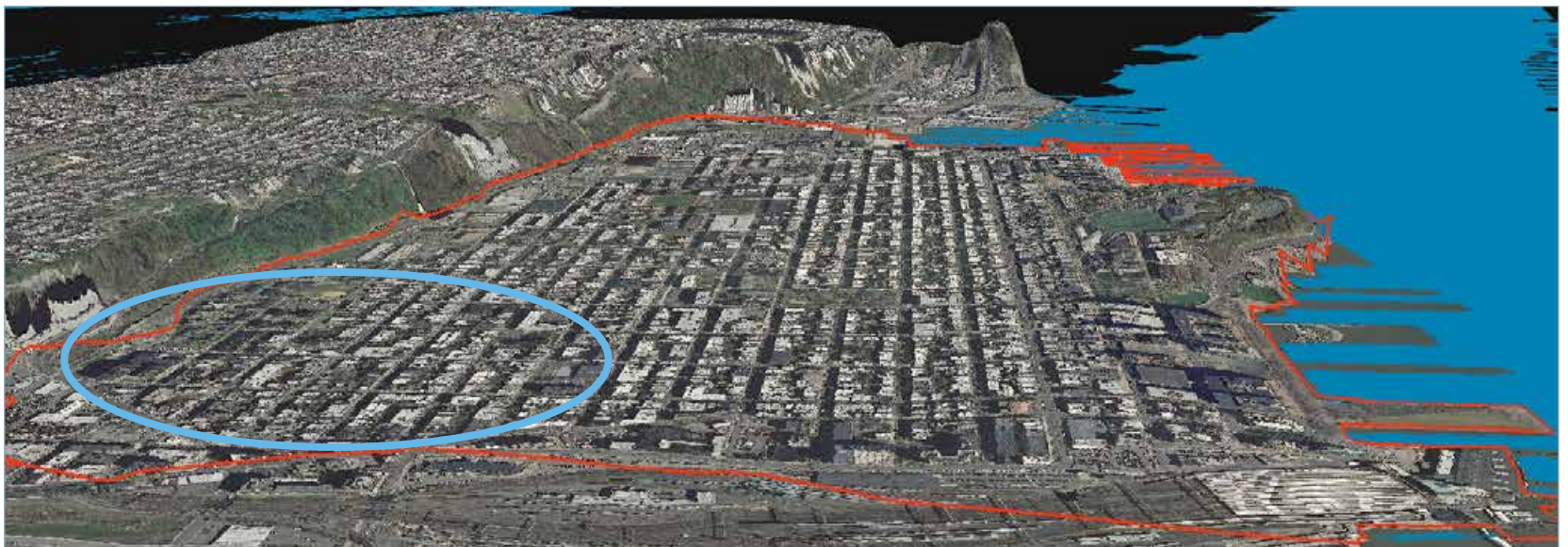
Hoboken’s topography lends itself to flooding. To the left, the New Jersey Palisades serve as a barrier along Hoboken’s western border, and the Hudson River waterfront is higher than the southwestern area of the city (circled), so water tends to pool there.
